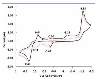
**Figure 5.** Cyclic voltammograms of  $[1-H_2]^+$  in fluorobenzene. For the black trace (solid line), the initial scan direction was positive. For the red trace (dotted line), the initial scan direction was negative. Conditions: 1.0 mM  $[1-H_2]^+$ ; scan rate, 100 mV/s; electrolyte, 0.2 M n-Bu<sub>4</sub>NBAr<sup>F</sup><sub>4</sub>; 1.0 atm H<sub>2</sub>.
