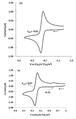
Figure 4. (a) Cyclic voltammogram of 1-Cl (1 mM) and (b)  $[1]^+$  (1 mM). Conditions: scan rate, 100 mV/s; electrolyte, 0.2 M n-Bu<sub>4</sub>NB(C<sub>6</sub>F<sub>5</sub>)<sub>4</sub> in fluorobenzene.
