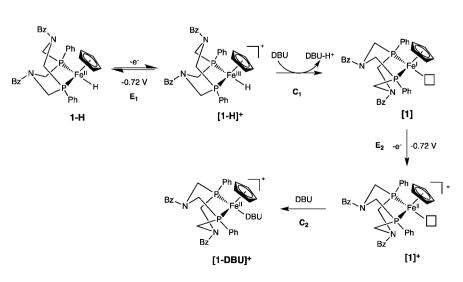
conformation, the pendant base is positioned to participate in  $H_2$  cleavage with a low activation energy.
