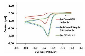
**Figure 7.** Cyclic voltammogram of **1-H** (0.5 mM) in the absence of DBU (red trace), in the presence of DBU (5 equiv, blue trace), and in the presence of DBU (5 equiv) and H<sub>2</sub> (1.0 atm, green trace). Conditions: scan rate, 100 mV/s; electrolyte, 0.2 M n-Bu<sub>4</sub>NBAr<sup>F</sup><sub>4</sub> in PhF.
