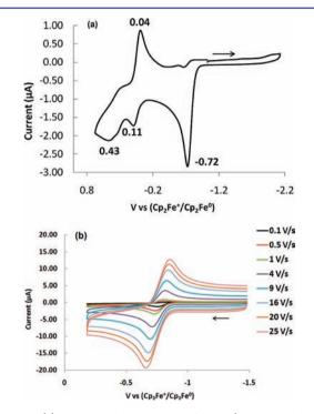
**Figure 6.** (a) Cyclic voltammogram of **1-H** (1.0 mM solution). Conditions: scan rate, 100 mV/s; electrolyte, 0.2 M n-Bu<sub>4</sub>NBAr<sup>F</sup><sub>4</sub> in PhF; under Ar (1.0 atm). (b) The oxidation wave at -0.72 V recorded at scan rates from 0.1-25 V/s.
